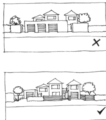
Figure 5: Eliminating blank walls and rows of garages creates a more pleasant streetscape.
